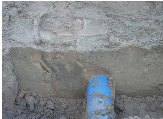
Figure 5. Borehole filling with material of low conductivity caused by problems to remove the cuttings
